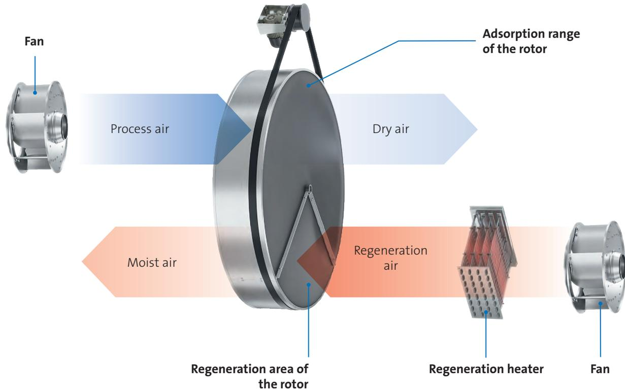
Desiccant drying - typical principle of operation
