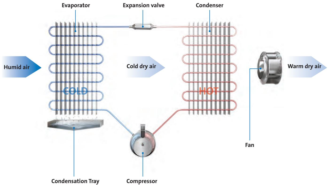
Condensing dehumidification — typical principle of operation
